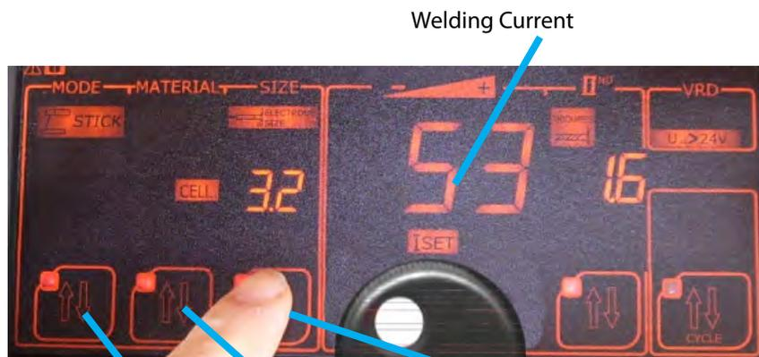
A - Select STICK    B - Select electrode type    C - Select electrode size
