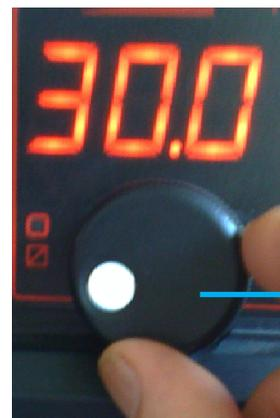
C - with the main knob adjust the current level or the basic material tick
