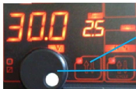
The main knob allows arc setting between -20 (short) and +20 (long). The -0- value correspond than to the pre-set synergic value.
