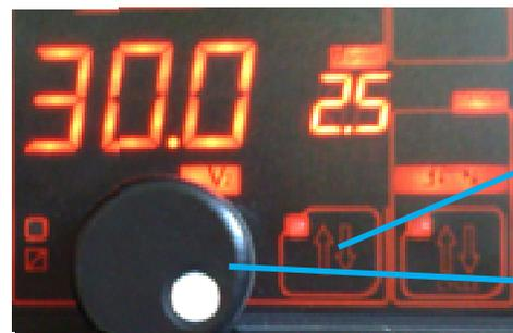
A - press until arc lenght led light on
